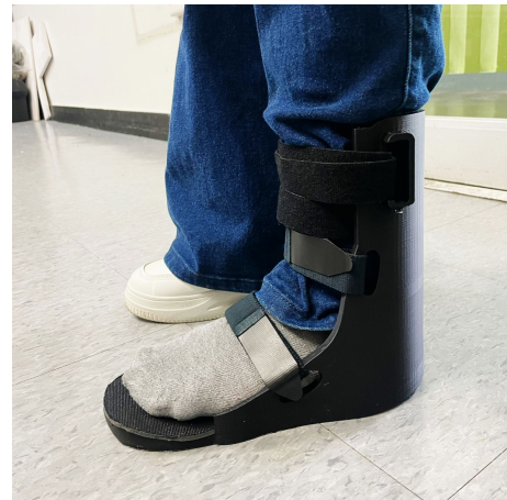
Fig. 5. Printed boot test inside the laboratory.
